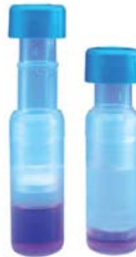
Fig 3. The Mini-UniPrep filter on the left is shown with fluid in the chamber. On the right, the filter plunger is shown compressed with the sample ready for analysis.
