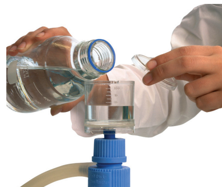
Fig 1. Sample is poured into monitor unit and filtered. (Workflow continued on next page)
