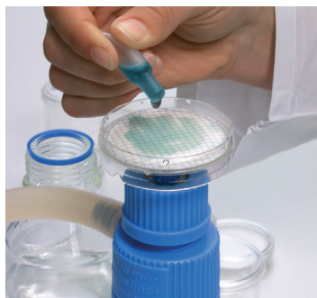
Fig 3. Microbiological media is added to membrane.
