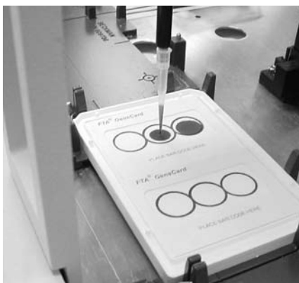
Fig 3. Blood sample being applied to Gene Card Tray on a Biomek™ 2000.
