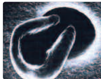
AN ERYTHROCYTE PASSING THROUGH A 2.5 \mu\text{m} PORE IN A TRACK-ETCHED MEMBRANE
